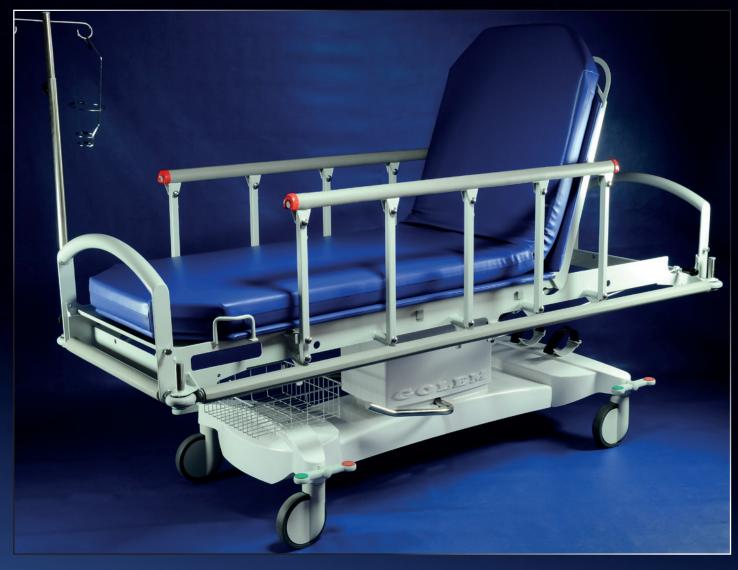
An optimal means for the transport of patients with a possibility of X-raying directly on the table. High-quality travel wheels Ø 150 mm with two central brakes; leading wheels for straight direction. Two-part working surface of  $630 \times 1965$  mm, back segment adjusted manually using by gas spring, from 0° to +75°. Outside dimensions (clearance profile)  $760 \times 2070$  mm.
